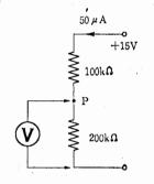
of -25%. For a low sensitivity tester, the error will be -63% reading it 3.73V.
